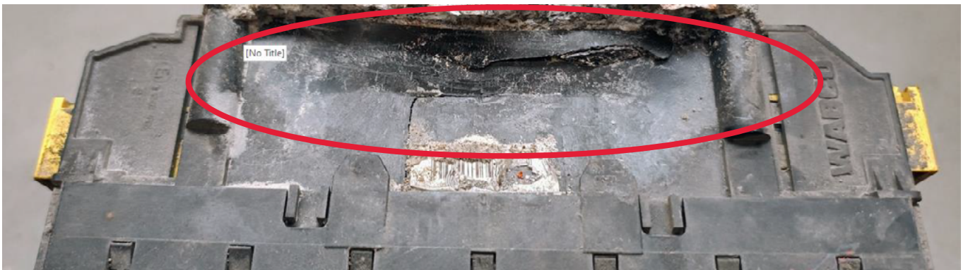
Deformed / distorted ECU
