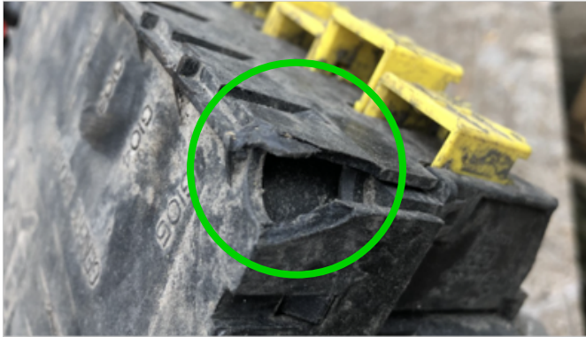
Missing small plastic parts on ECU
