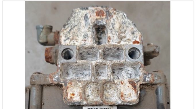
Corrosion on body
