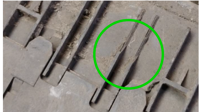
Damaged ribs on the ECU Cover
