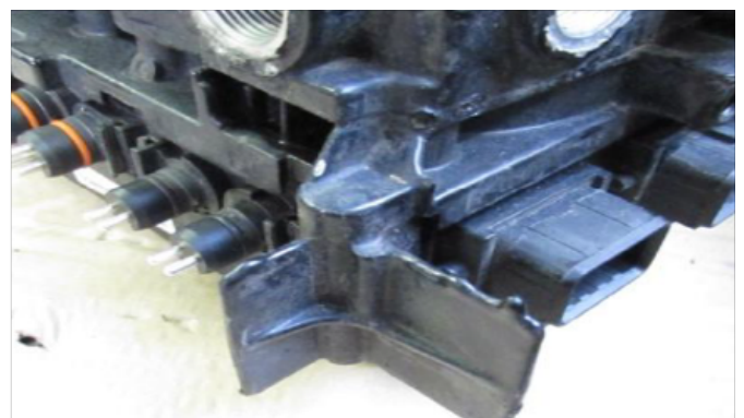
Damaged external cover elements
