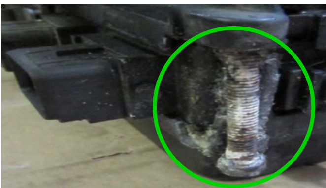
Damaged external cover elements
