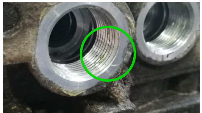
Damaged ports, scratches on the sealing surface
