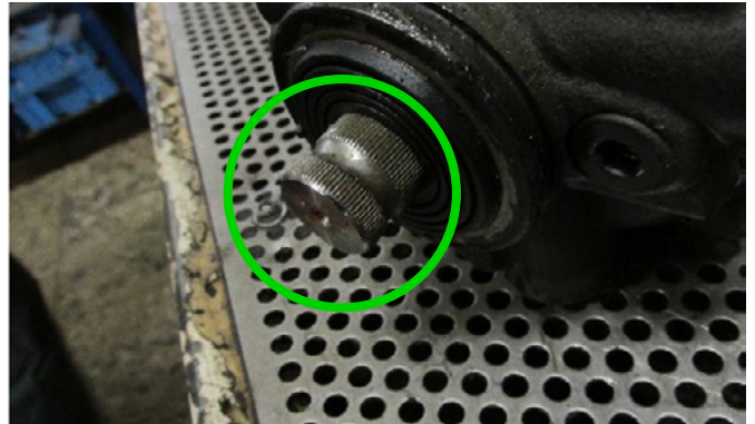
Valve without damages
