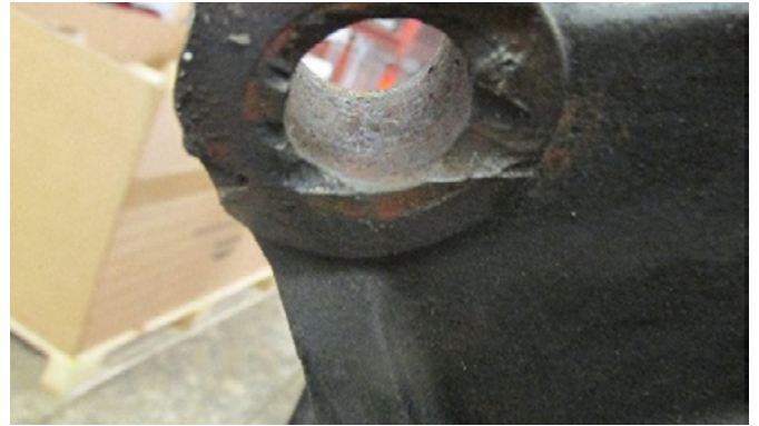
Unprofessional disassembly – damaged housing
