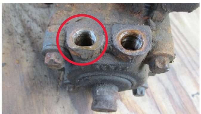
Damage valve cover
