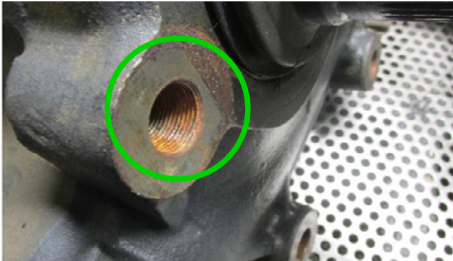
Thread without damages
