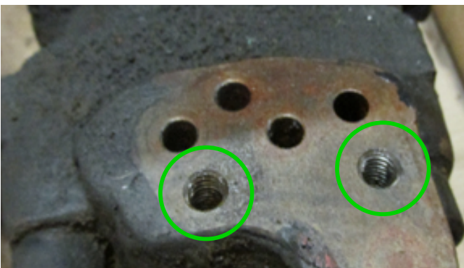
Thread without damages
