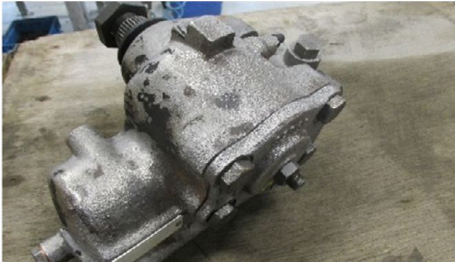
No or small signs of rust
