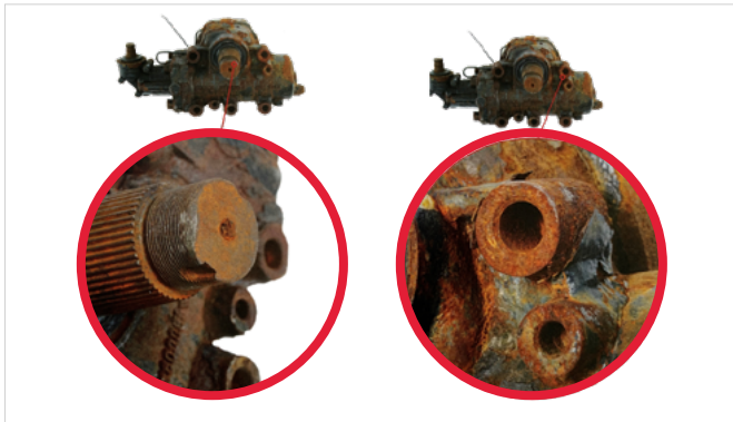
Heavy rust on marked area
