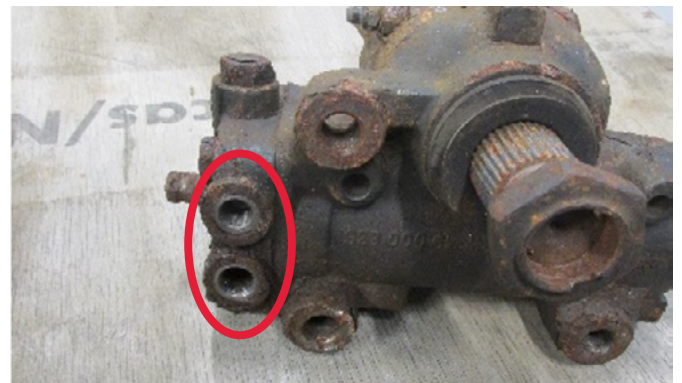
Transporter plugs missing
