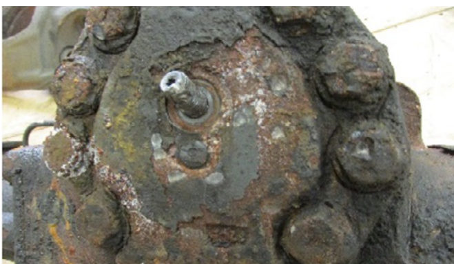
Damage side cover
