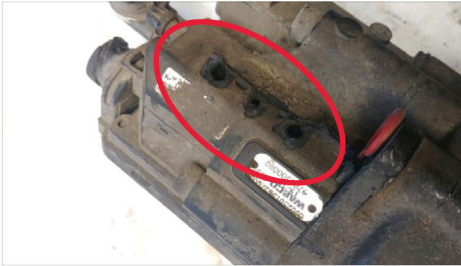
Serious damages of a solenoid valve box. Missing material.
