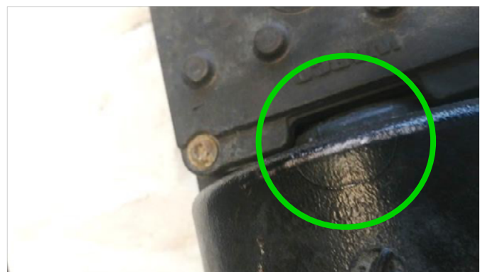
Scratches on external surface
