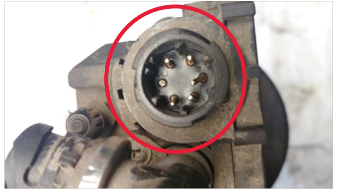
Missing, bent pins or corrosion in the connector.
