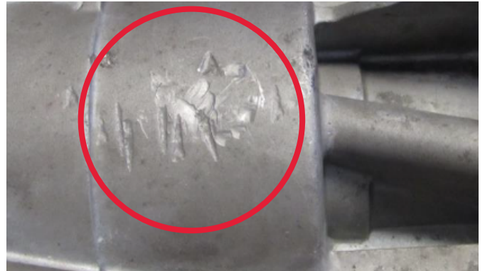
Significant signs of hit on external surfaces
