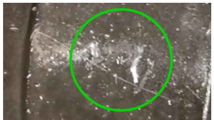
Scratches on external surface
