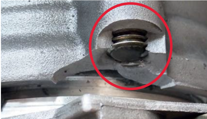
Serious damages to the body. Missing material
