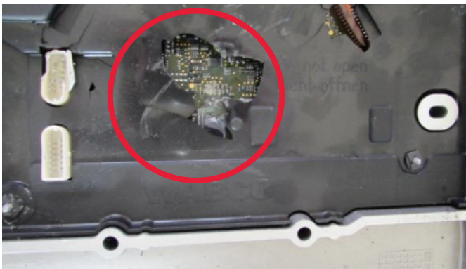
Hard damages of ECU cover
