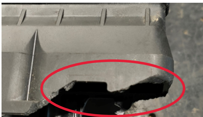
Serious damages on ECU
