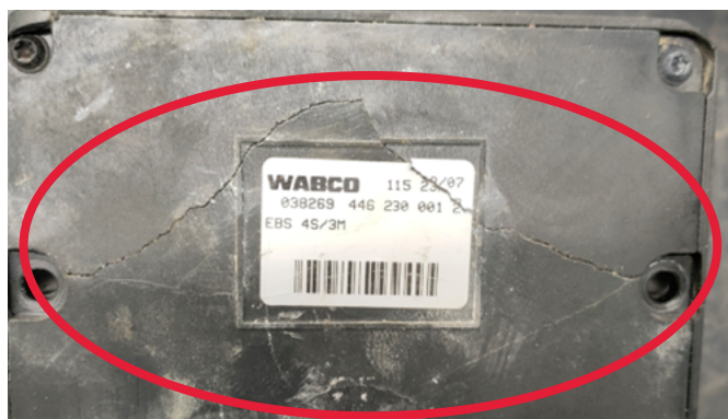
Serious damages on ECU
