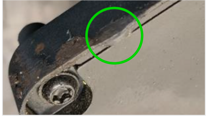
Small mechanical damages on ECU
