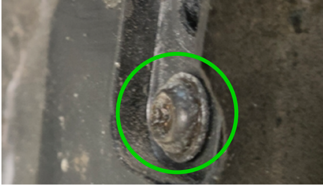
Missing material on ECU
