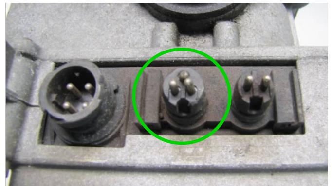
Bent Pins, Scratches on connector (generation 1, 480103XXXX)
