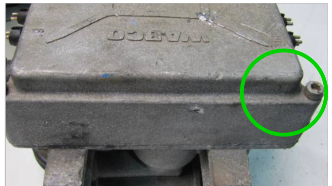
Cutted, damaged or missing cover flips
