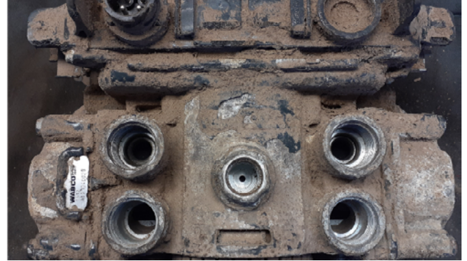
Surface contamination, dirt.
