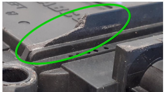
Missing small parts of plastic cover
