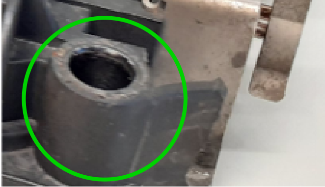
Broken rib of plastic cover
