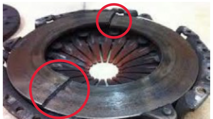
Pressure plate broken
