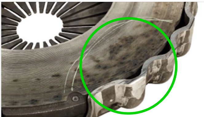
Blue metal through overheating
