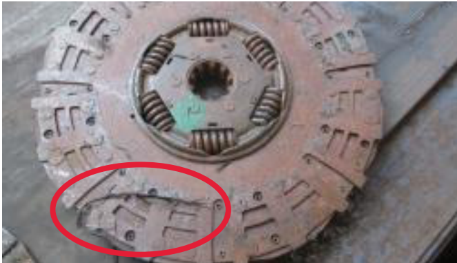
Clutch disc is bent or broken. Hub is broken. Damper is broken.
