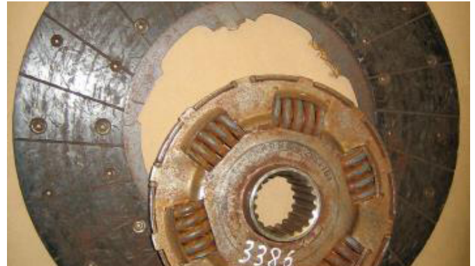
Clutch disc is bent or broken. Hub is broken. Damper is broken.
