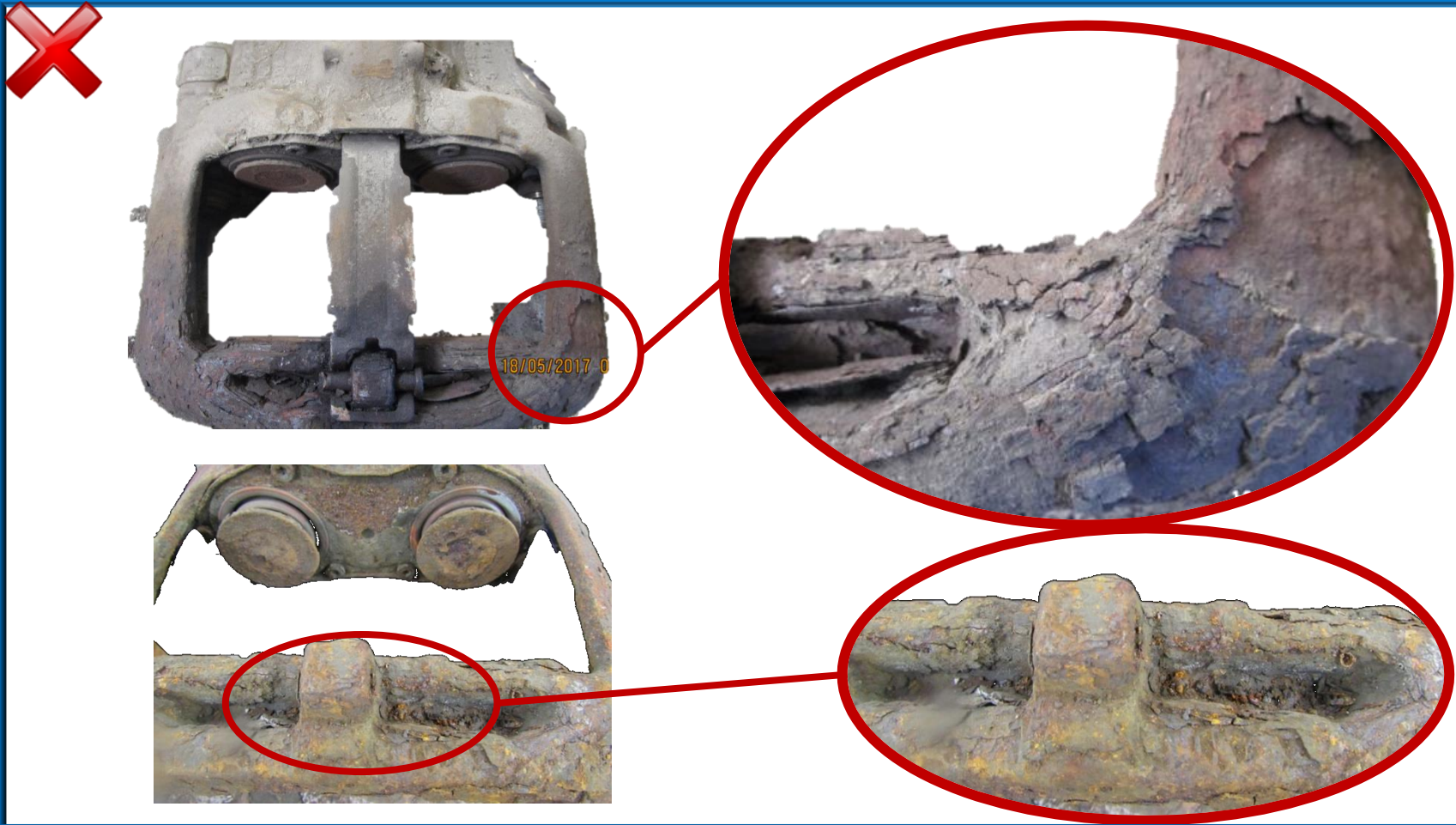
Heavily corroded calipers
