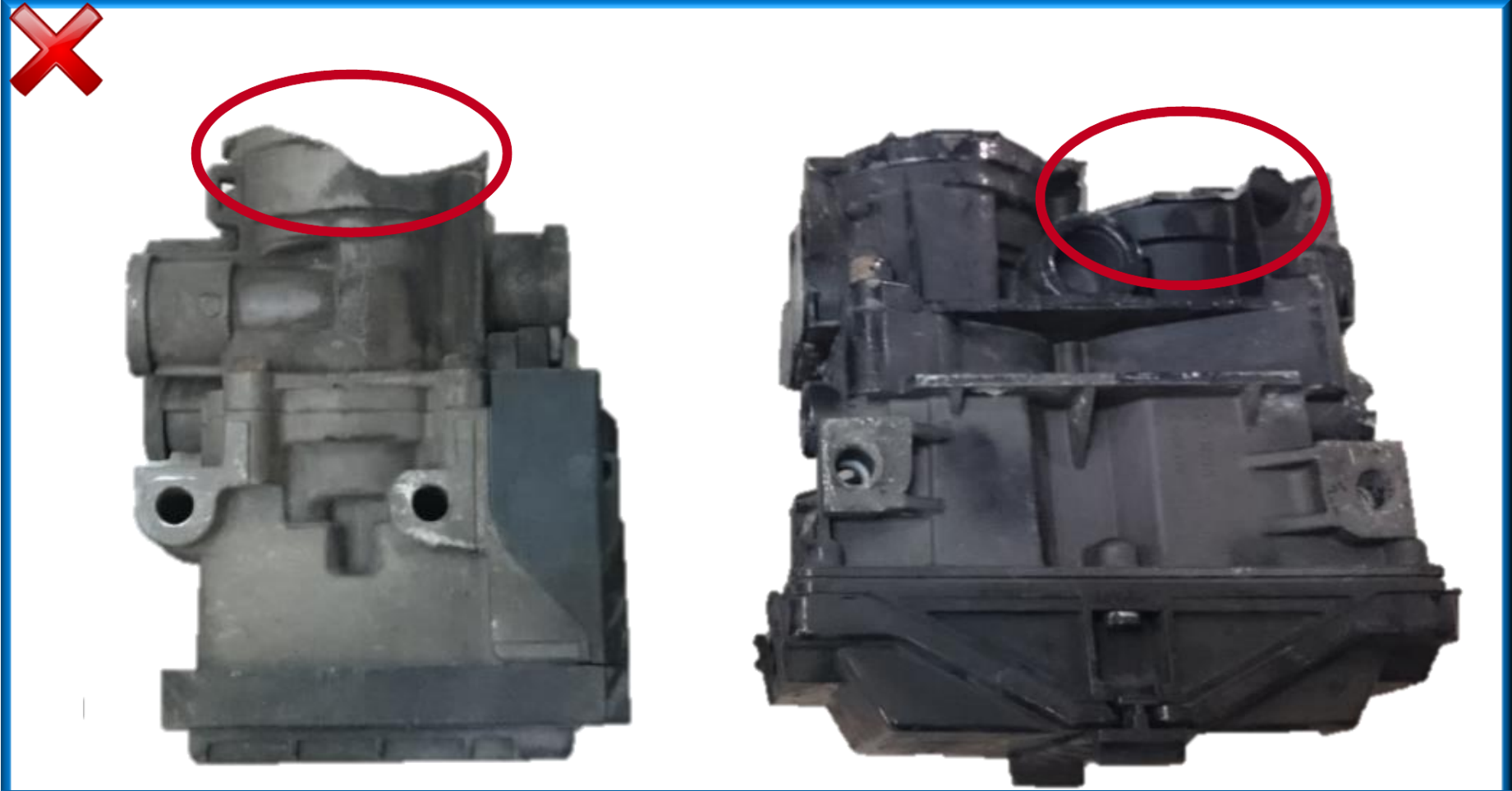
Heavily damaged housings caused by non-operational use
