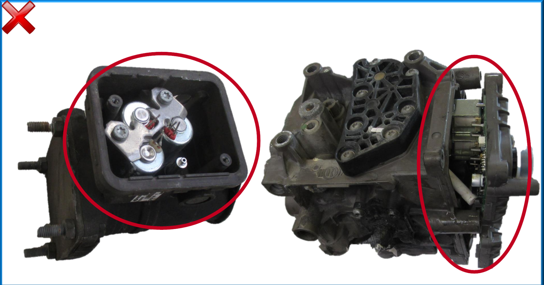
Missing housing / Disassembled condition
