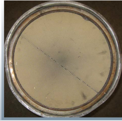
Cracked filter due to being dropped. Un-repairable.
