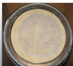
Massive failure due to uncontrolled thermal event while on the truck. Blue area is all black holes. Filter is no good.
