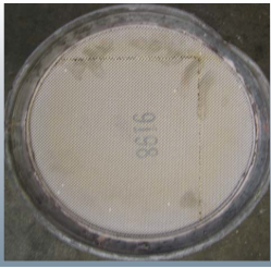
Cracked filter due to being dropped.
