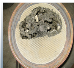
Defect: High pressure reading on the air flow test bench but nothing visible to the eye. When we broke the filter apart to see what was wrong, we found it melted inside.
