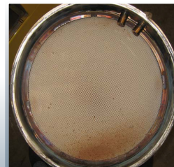
Rust or Chemical Stain Fully recoverable with pneumatic cleaning.
