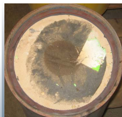
Plastic melted on filter face.
