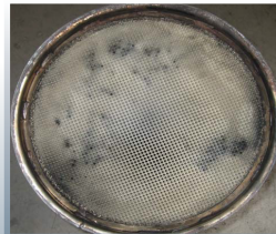
Black holes a little harder to see—too many, Filter no good (as viewed from clean side).
