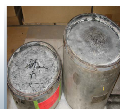
Uncontrolled thermal regeneration on a truck. Filter and catalyst destroyed.
